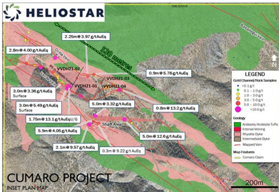
Figure 2: Detailed sampling and mapping from the Verde Vein Corridor with selected samples highlighted
