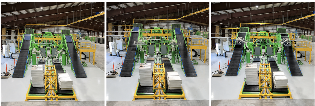
Comstock Metals’ robotic arms feeding solar panels onto conveyance system.
